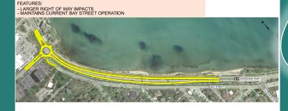
CONCEPT: CONSTRUCT ROUNDABOUT AND CLOSE BAY STREET ACCESS AT M-72 FEATURES:
