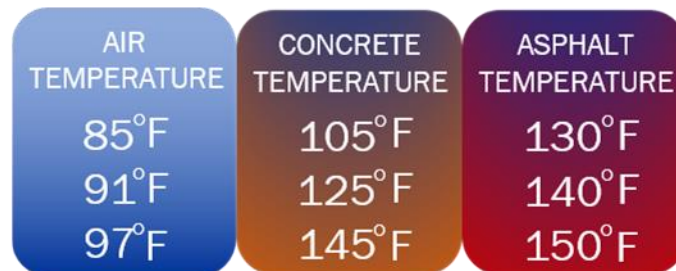
Figure 5. Impact of Heat on Concrete and Asphalt
