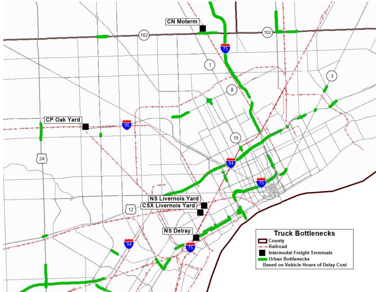
Figure 20. Intermodal Terminal Highway Access Bottlenecks
