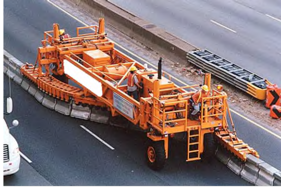
Exhibit 6-8: Moveable Barrier Operation
