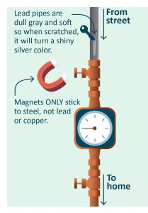
To determine what material your service line is made from, you can do a scratch test and magnet test on that side of your water meter. To test your home's plumbing, you can do the scratch and magnet test on the plumbing on the other side of your water meter.
