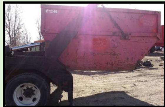
The picture on the left is an example of containers stored in a storm-resistant shelter. The picture on the right shows an acceptable method for loading a container onto a truck for transport. Notice the container is not tipped during the loading sequence.
