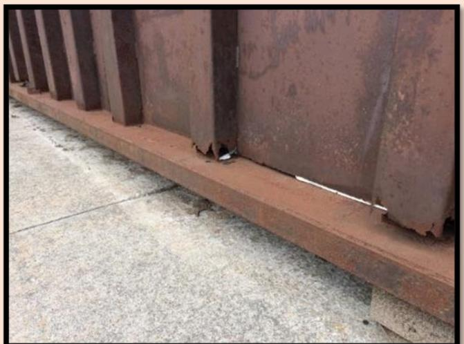
The picture on the left identifies leaking hydraulic oil issues and the picture on the right shows a non-leak-tight compactor due to rusting conditions.
