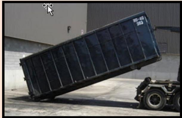
The picture on the left identifies spilled materials at the container storage area and the picture on the right shows a roll off container being tipped during loading. Tipping roll off containers with swinging rear doors typically allows fluids to be discharged from the container.
