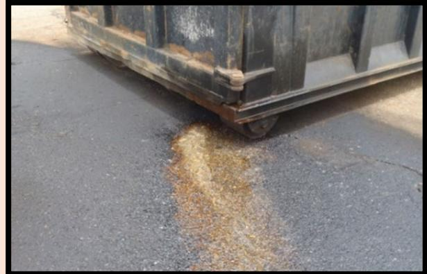
The picture on the left identifies a roll off container with a swinging rear door. These types of containers will typically allow fluids to be released from the container. The picture on the right shows a container that is leaking fluids.
