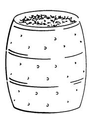
A Plastic 55 gallon drum can be turned into an effective compost bin in a few simple steps. Merely cut off the top and bottom of the barrel with a sabre saw and cut a series of 2" to 3" holes in the sides for aeration.
