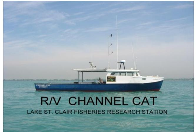
The research vessel *Channel Cat* is a steel hulled fish tug designed for a trap net fishery operation, similar to the Lake Erie trap net tugs. She was built for the DNR in 1968 by the Maybee Boat Company. Since that time, the *Channel Cat* has served as a work platform for Great Lakes fisheries research. The *Channel Cat's* home port is the Michigan Department of Natural Resources Lake St. Clair Fisheries Research Station located at the mouth of the Clinton River on Lake St. Clair.
