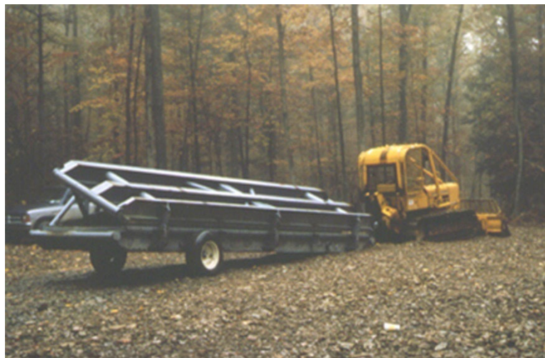
Figure 19. A Portable Folding Metal Bridge.
