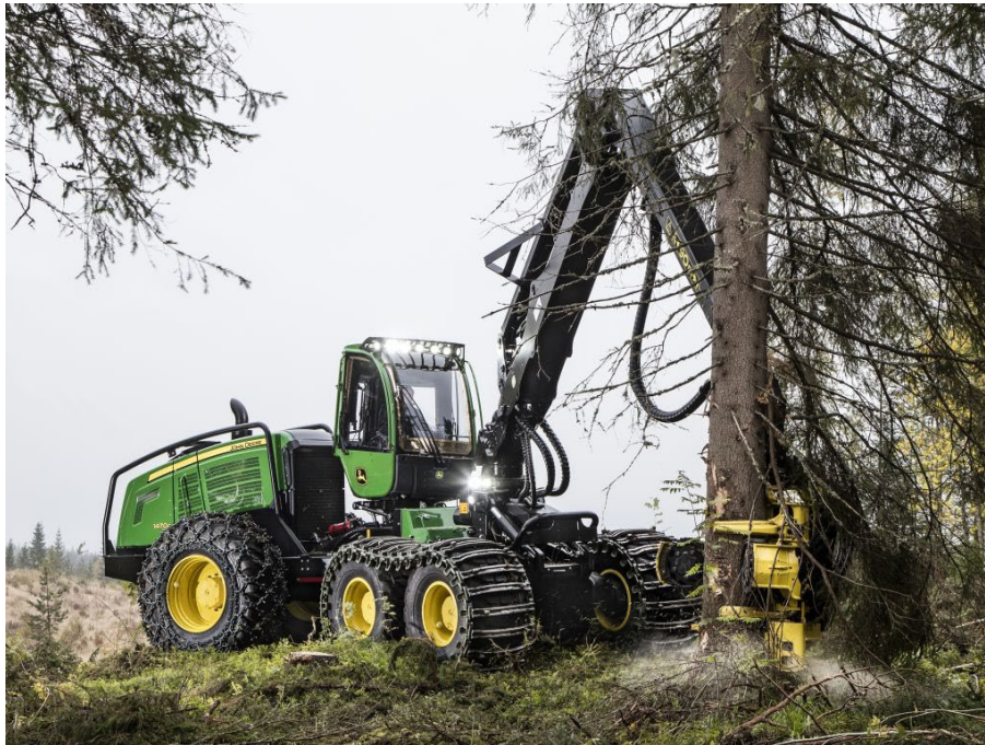
Figure 23. John Deere G Series Harvester with High Floatation Tires & Tracked Wheels.
