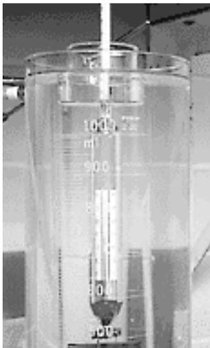
The hydrometer is allowed to float in the solution to be tested. The greater the specific gravity of the solution, the less the hydrometer will sink into it. The specific gravity of the solution is read on the scale at the surface of the solution.
