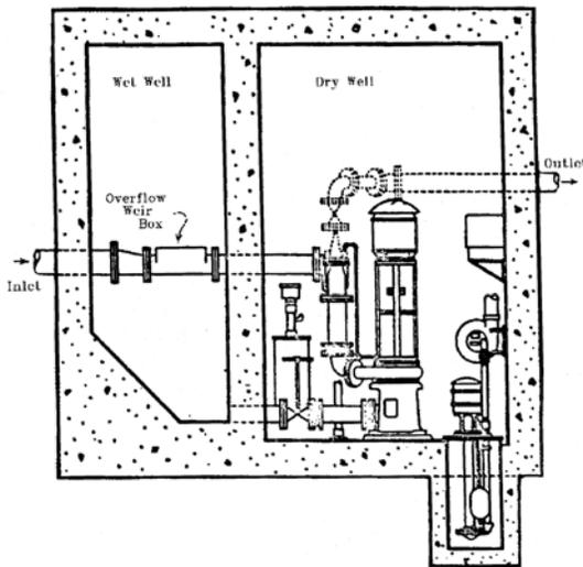
Figure 2 - Pump in dry pit. Motor on top.
