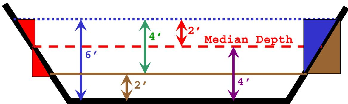
Lagoons are designed to utilize only the top four feet for storage. The bottom 2 feet are allocated for sediment. **Median depth** is 1/2 the depth of the water considered for storage. For this example the median depth is 4 feet from the bottom or two feet from the top.
