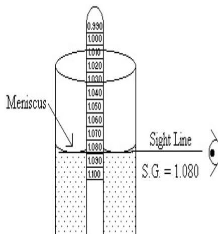
Since the hydrometer is calibrated at 20 degrees C, specific gravity should be determined on solutions which are at room temperature.
