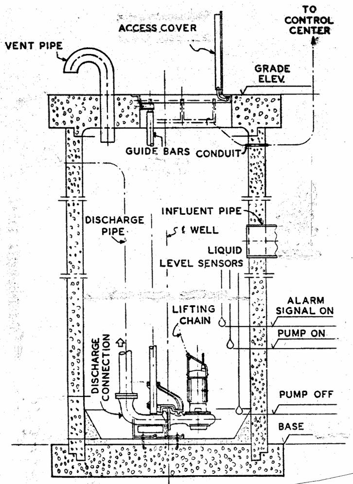
Manhole Used as Wet Well Station (Figure 1)
