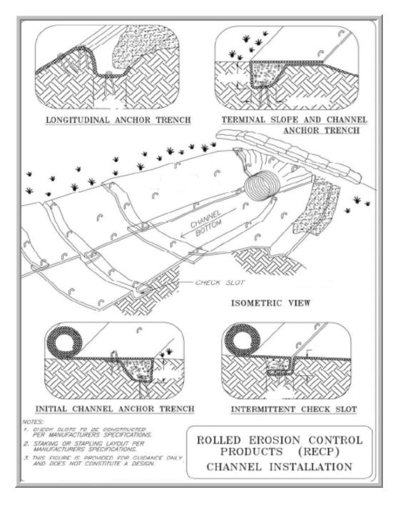
Source: Ontario. Rolled Erosion Control Product (RECP) BMP 11.
