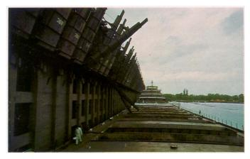
The iron industry has come a long way since the first iron was smelted back in the mid 1800s. The ore boat (above and below) is loading at a special dock at Marquette. Rail cars above the dock dump their loads into the chutes for speedy loading. A world leader in iron production for years, Michigan continues to rank among the top 10 areas, although one of our major ranges is no longer mined.
